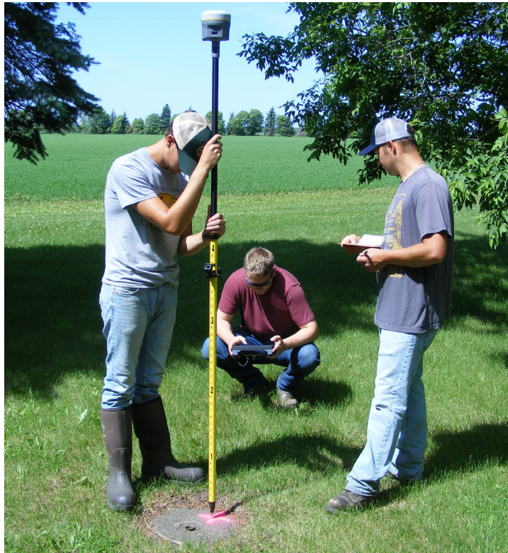
From left: Matt Sorvig, Pennington SWCD resource technician; Zach Foley, Technical Services Area 1 technician; and Peter Nelson, Pennington SWCD water plan coordinator, close a bench mark shot on a GPS survey they completed for a grade stabilization project on a Pennington County farm.
